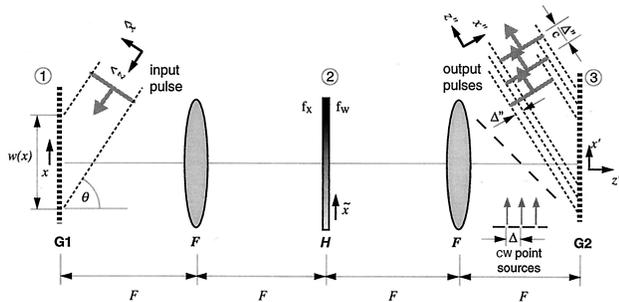
Fig. 1. Structure of the parallel-to-serial transmitter. cw writing beams emanating from point sources separated by  $\Delta$  propagate from right to left, coupled in by a beam splitter (dashed line). An incident short pulse propagates from left to right, with the spectrum spatially dispersed at plane 2 (by a grating in plane 1), where a real-time 4WM process mixes the cw interference (with reference source not shown) and the pulsed spectrum.
