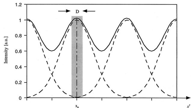
Fig. 5. Intensity output of diffracted data points. Spots are displaced by  $x_0$ , a distance that guarantees a signal-to-cross-talk ratio of 20 dB. The shaded area corresponds to light intensity gathered by a detector of width  $D$ .
