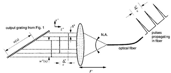
Fig. 4. Coupling output pulses of transmitter into an optical fiber. The output pulses, of the size  $w''(x)$ , are delayed by  $\Delta''/c$  and laterally shifted by  $\Delta''$ . Lens  $F'$  couples the pulses into a fiber, where the lateral shift information is lost.
