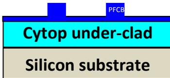
Finally we removed the SiO<sub>2</sub> hard mask using *SiO<sub>2</sub> etch* recipe as we did before. It is important to mention that removing the SiO<sub>2</sub> etched only 30nm PFCB layer as can be seen in figure 4.13 where SiO<sub>2</sub> etch was applied on a half covered PFCB layer for duration of 1 min.
