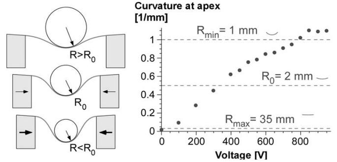
Fig. 3. (Left) Reflecting membrane stretched between two actuators. As the actuators move towards each other, the membrane buckles resulting in a curved region at the center. (Right) Measured curvature versus applied voltage on the piezoelectric actuators.
