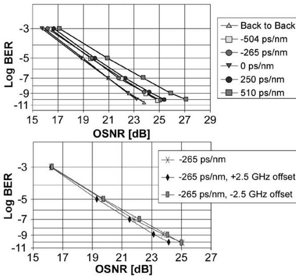
Fig. 7. (Top) Receiver sensitivity curves for different amounts of fiber dispersion in the link. The legend dispersion values are of the inserted fiber, and the TDC dispersion setting is the opposite of that. (Bottom) Sensitivity curves for laser transmitter misalignment with respect to filter center.
