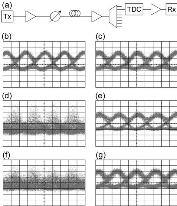
Fig. 6. (a) Setup for characterization of TDC performance in receiver sensitivity experiments. (b) Back-to-back performance of transmitter and receiver. (c) TDC inserted in a transmission link. (d) SMF inserted, generating 425-ps/nm dispersion. (e) TDC compensating 425-ps/nm dispersion. (f) DCF inserted, generating -504-ps/nm dispersion. (g) TDC compensating -504-ps/nm dispersion.
