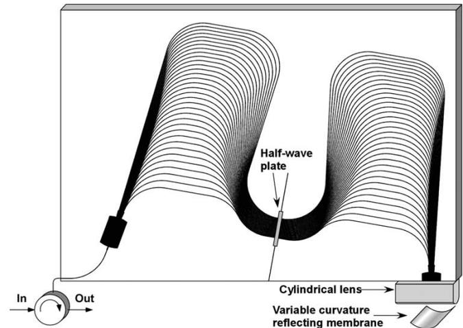
Fig. 1. Schematic layout of the optical TDC, comprising of a WGR, collimation lens, deformable mirror, and a circulator.
