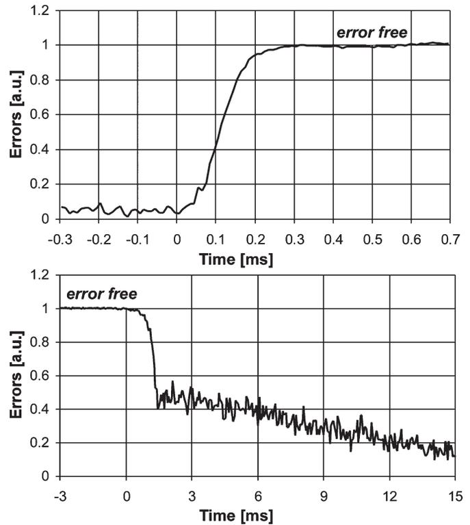
Fig. 8. TDC response time measurements performed with receiver error counts. (Top) Fast response to increasing voltage (dispersion). (Bottom) Slower response to decreasing voltage (dispersion) with two time constants visible.
