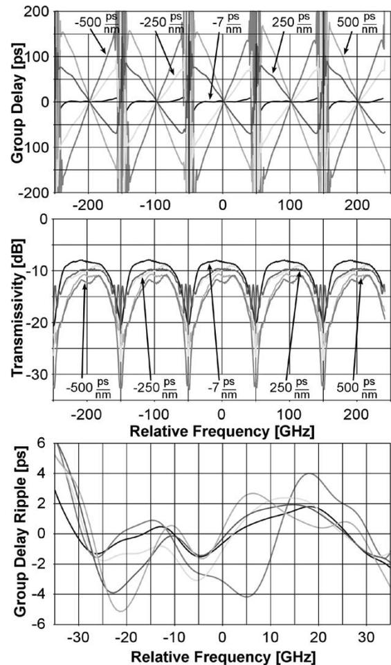
Fig. 5. (Top) Group delay versus frequency. Different slopes are observed, corresponding to dispersion settings. (Center) TDC transmissivity versus frequency. Spectral narrowing is observed for larger departures from zero dispersion. Passband and dispersion settings are repeated at 100-GHz FSR. (Bottom) GDR for all dispersion settings at one particular channel. Ripple is bounded by  $\pm 6$  ps over  $\pm 35$  GHz from channel center.
