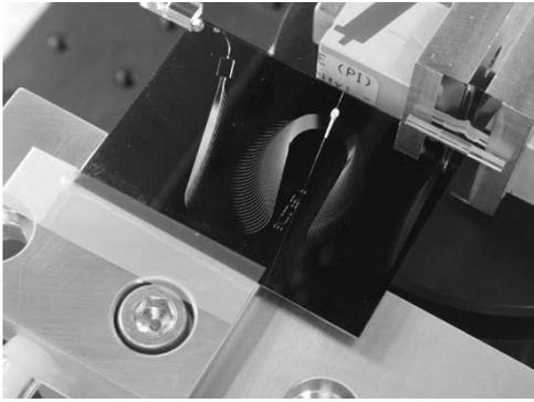
Fig. 4. Photograph of TDC showing the PLC, the attached cylindrical collimation lens, and the deformable Mylar mirror next to lens. The physical size of the PLC is 30 mm  $\times$  50 mm.
