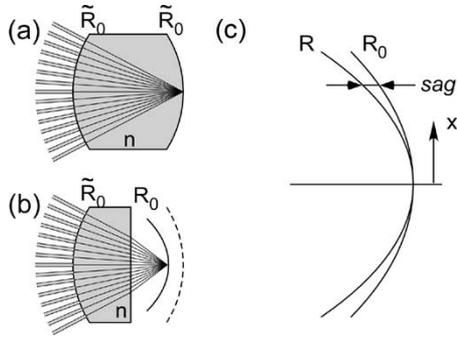
Fig. 2. (a) Free-space region as normally implemented inside a PLC. (b) Free-space region is cut and light propagates in air. The zero-dispersion curvature and location of the second surface of free-space region changes in air. (c) Adjusting the surface curvature of the membrane results in spatially varying sag values, which are approximately quadratic.
