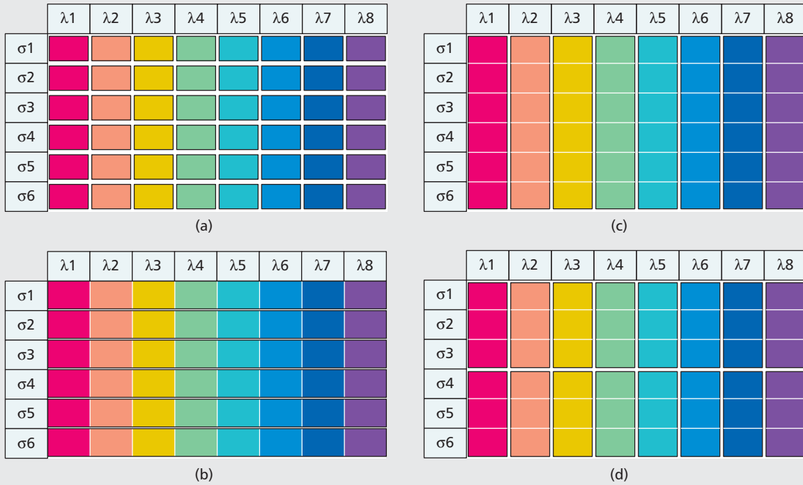
Figure 2. Parsing the fiber’s SDM and WDM channels for switching, where space modes ( \sigma_1, \dots, \sigma_M ) and wavelength channels ( \lambda_1, \dots, \lambda_N ) are fully utilized: a) space-wavelength granularity (each mode/wavelength channel can be independently switched); b) space granularity (switching performed on a mode basis across all wavelengths); c) wavelength granularity (switching performed on a wavelength basis across all modes); d) fractional space-full wavelength granularity (switching performed on a wavelength basis and spatial mode sub-groups).
