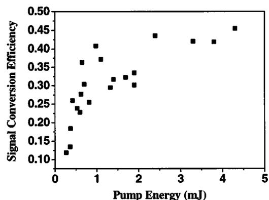
FIG. 5. Signal conversion efficiency vs pump energy (compensated for Fresnel and filter losses).
