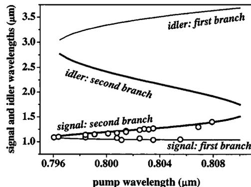
FIG. 1. Phase matching condition in PPKTP with period of 27.1  $\mu\text{m}$  pumped by a  $\sim 12$  nm chirped Ti:sapphire laser. Open circles are experimental data. The curve was calculated from Sellmeier's coefficients in Ref. 10.
