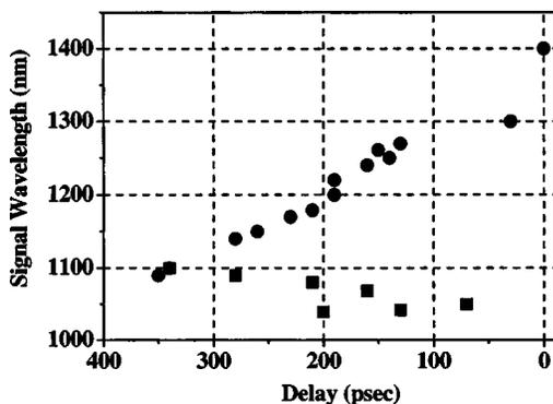
FIG. 3. Delay between the output from the Si photodiode and the signal from the InGaAs photodiode as a function of the wavelength. Lower signal's lobe—squares. Upper signal's lobe—circles.
