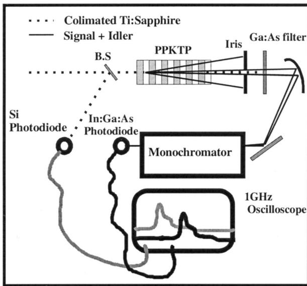
FIG. 2. Experiment setup. The spectrum is scanned by a monochromator and InGaAs photodiode. The chirp was measured by measuring the delay between the two photodiode signals, as a function of the wavelength.
