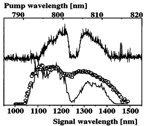
FIG. 4. Spectrum of the laser (upper trace) and signal (lower trace). Blocking some of the seeding spectrum in the regenerative amplifier creates the gap in the spectrum. The circles show the broadening of the spectrum due to noncollinear phase matching (taken without an iris). The continuous lower trace shows the signal spectrum when an iris blocks noncollinear beams. The intensities of the two spectra were rescaled.
