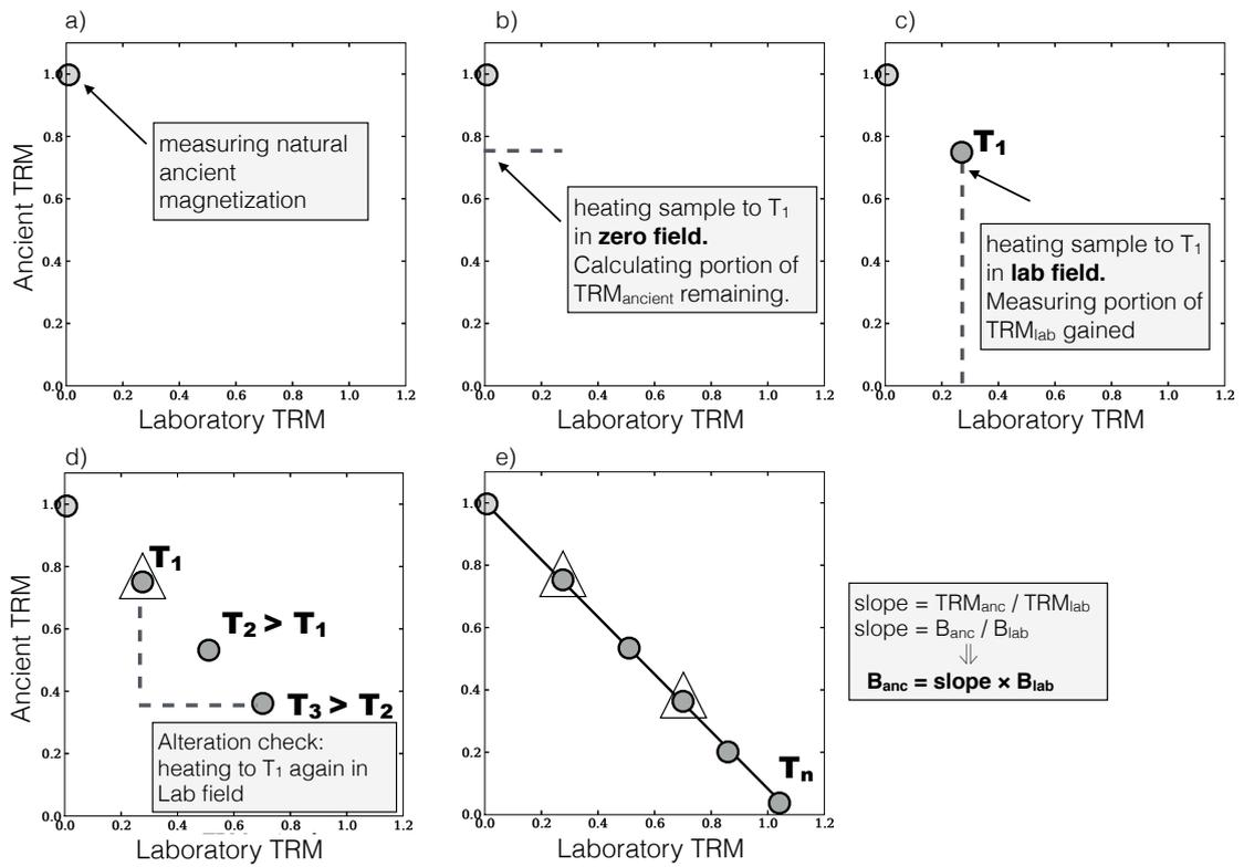
Figure 1: Schematic illustration of the Coe variant of the Thellier method (see text for details).
