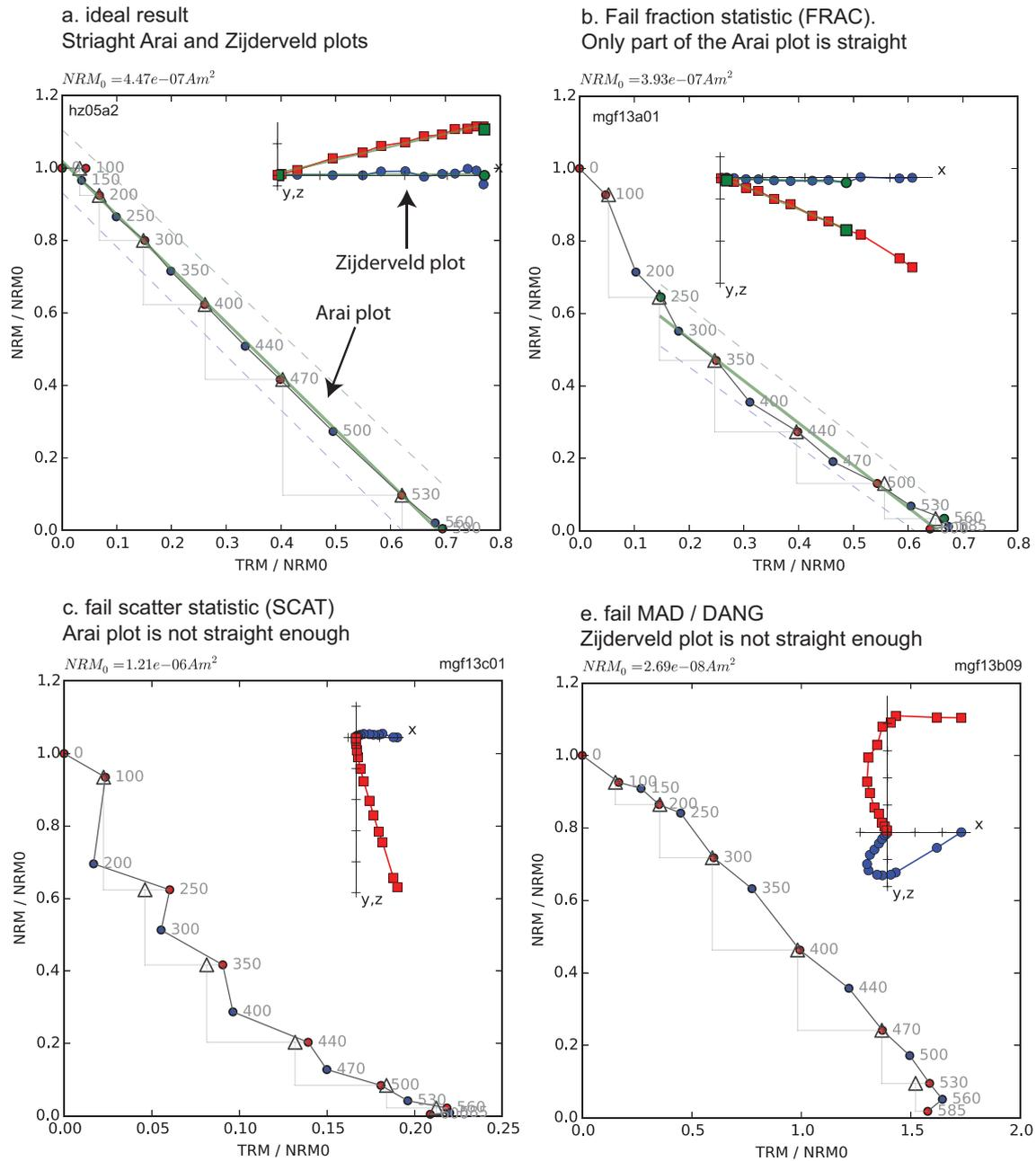
**Figure 2: Representative result showing Arai plots (see text) and orthogonal Zijdeveld plots (insets) of different pottery fragments. a) Ideal Arai and Zijdeveld plots showing straight line. Paleointensity can be calculated without ambiguity from the slope of the Arai plot. b-d) Examples of results that were rejected by our strict acceptance criteria: b) Arai plot is only partly linear; d) A scattered non-linear Arai plot; d) Non-linear Zijdeveld plots.**
